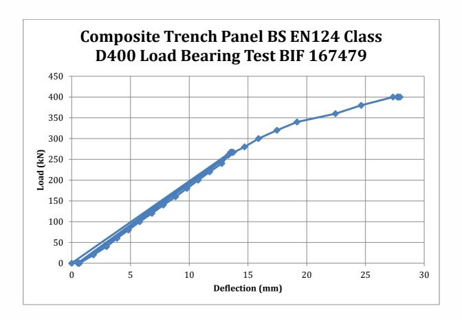
After the panel had passed the test it was reloaded until ultimate failure occurred at 481kN.
