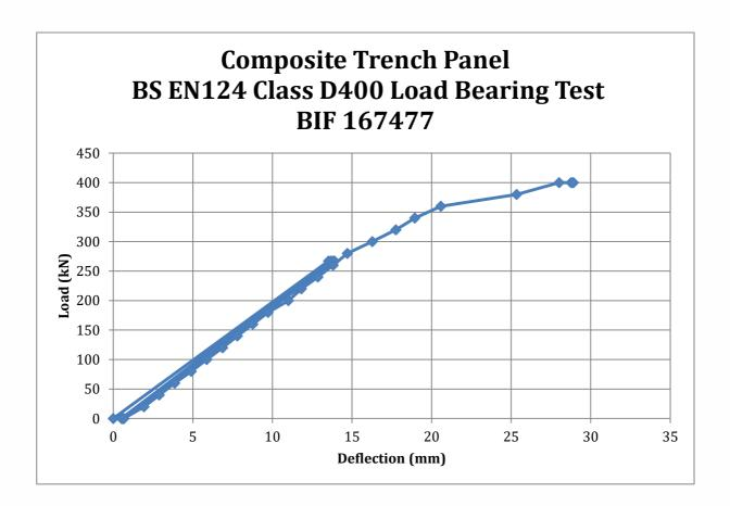
After the panel had passed the test it was reloaded until ultimate failure occurred at 475kN.
