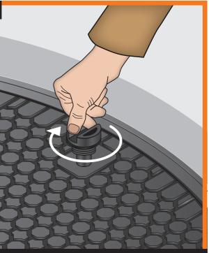
Clean out any debris in the lock housing, check and clean the security plug and seal before re-inserting.
