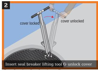
Insert lifting tool into the keyhole and turn the handle through 90° clockwise towards you to automatically disengage the cover lock.
