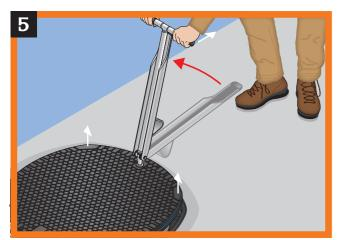
Fold back the foot plate into the lifting tool and lift cover from frame.
