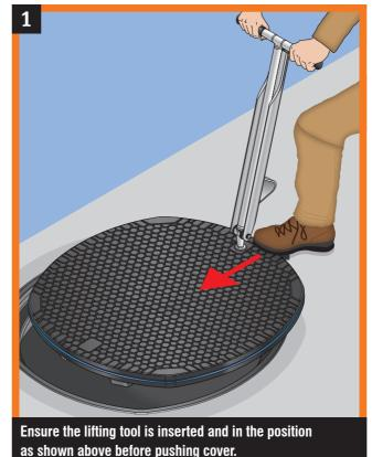
Push the cover back into the frame using your foot. Keep fingers away from cover/frame edge.
