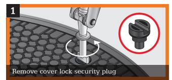
Insert lifting tool into cover lock security plug, turn through 90° anti-clockwise, unscrew and remove. DO NOT lose security plug.
