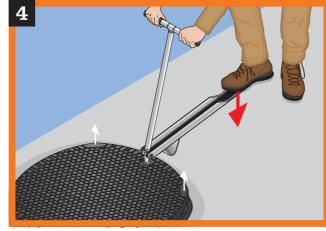
Press down firmly on the foot plate to release the cover from frame.
