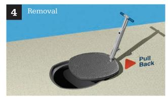
Fold back the seal breaker into the lifting tool. Lift the edge of the cover until free of frame. Pull the cover out of the frame.
